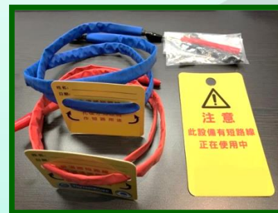
Figure 2 (8.1.c.iii): Temporary Jumper
